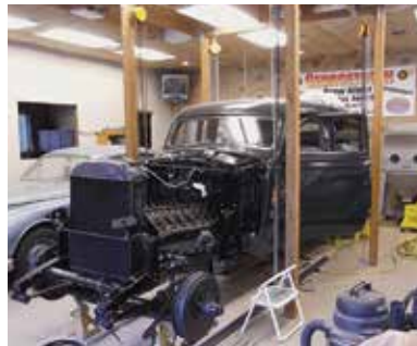
Aligning Hood to Body with Mock-Up of Upper Hood
