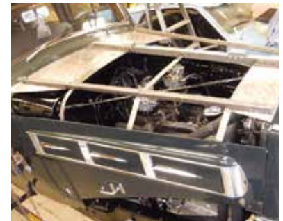
Aligning Hood to Body with Mock-Up of Upper Hood
