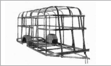
All-Steel framework - the girders and channel sections welded into one rigid integral unit.
