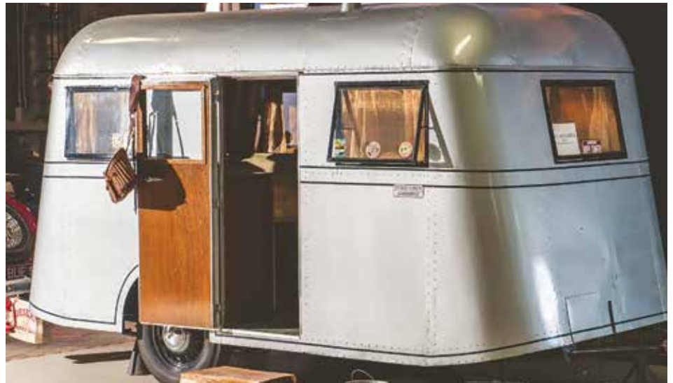
Travelodge Model C: Light, compact, full measure of utility to accommodate two people. Equipped with cooking stove, large double bed, china cabinets, drawers and wardrobe.
