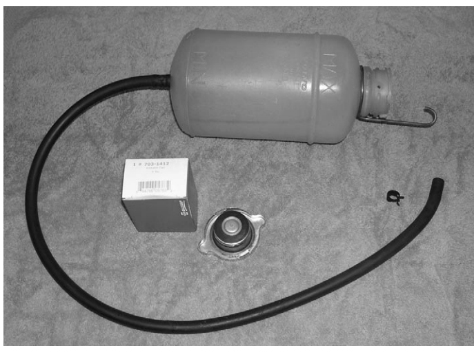
Installation supplies - tank, hose, clamp, pressure cap & NAPA box
